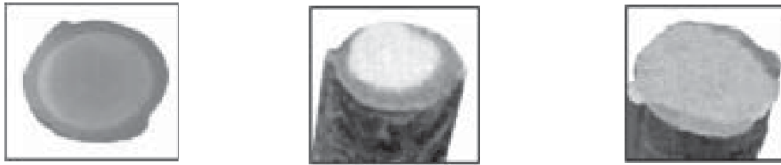
Figure 3 Macrographs of TMT rebars having different thicknesses of martensite rim
